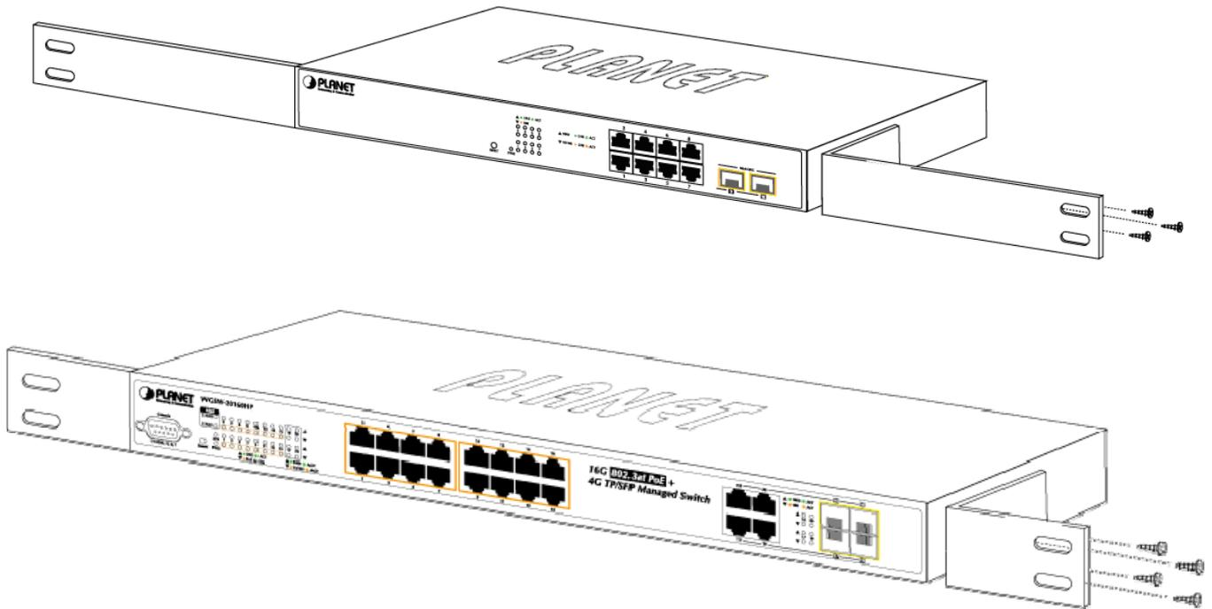
**Figure 2-22** Attach brackets to the Managed Switch.
