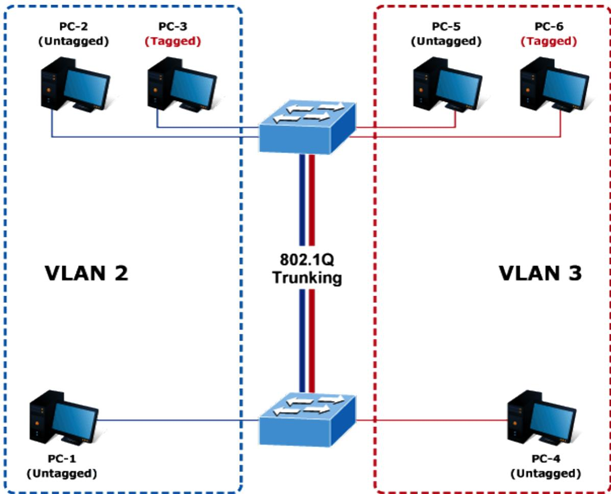
Figure 4-6-11: VLAN Trunking Diagram
