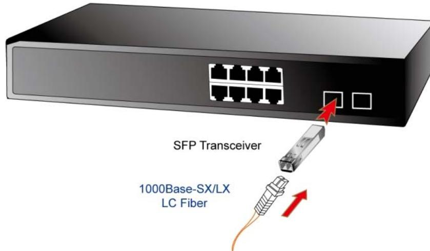
Figure 2-24 Plug-in the SFP transceiver
