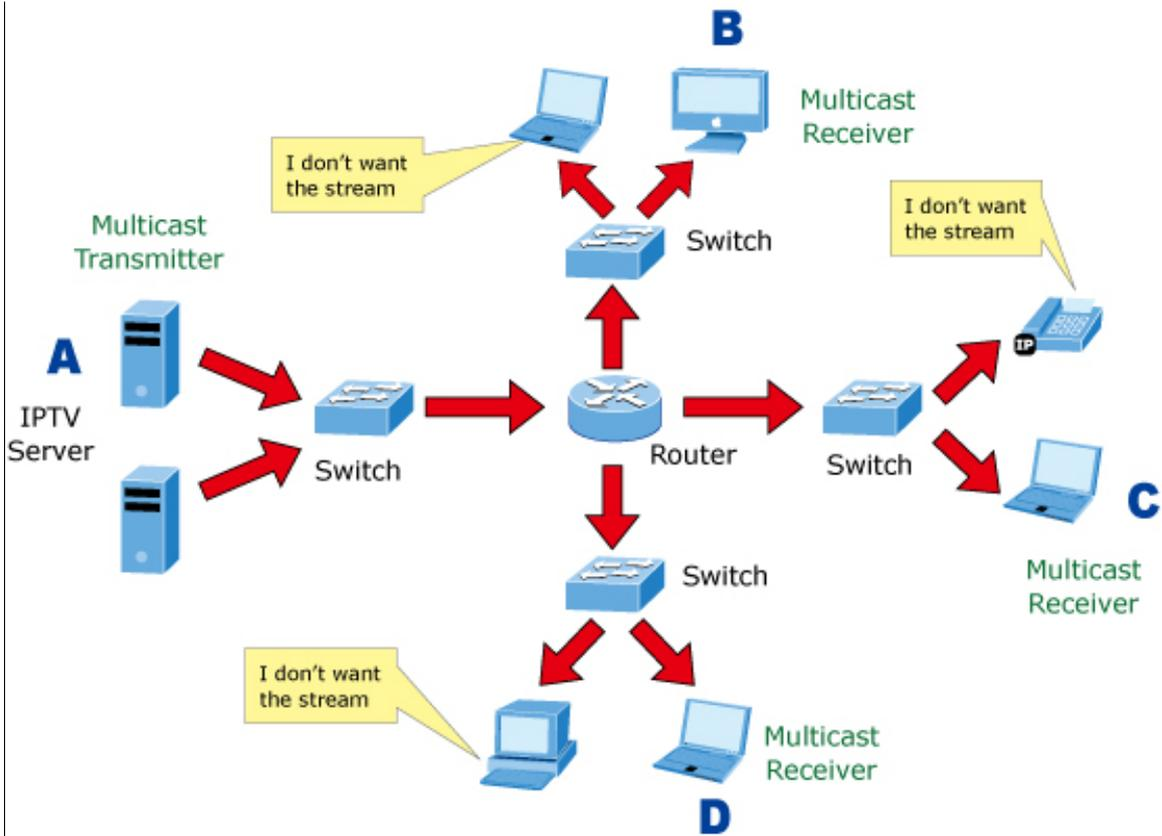
Figure 4-8-2: Multicast Flooding
