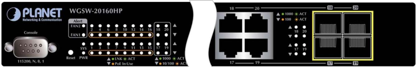
Figure 2-10 LED Panel of WGSW-20160HP
