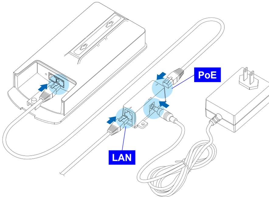
**Figure 2-1: Installing the ENS202**
